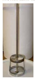
CUTDOWN II is packaged in 2 Parts: Part A and B, separate pails. You will need to supply a large enough pail (5-7 gal pail) and use it as your Mixing Pail. Pour Part A into mixing pail first, then add in Part B. Use a brush to scrape the material from each pail. Mix mechanically with a mix blade designed to mix low viscosity liquids, such as a Jiffy mixer. Mix thoroughly, at about 300 rpm, for 3 minutes until streak free. Avoid entraining air or mix until observable bubbling does not occur.
